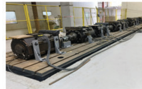
8 Traction Motor Set up for System Test
