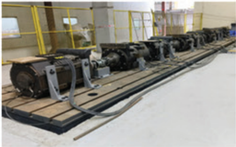
8 Traction Motor Set up for System Test
