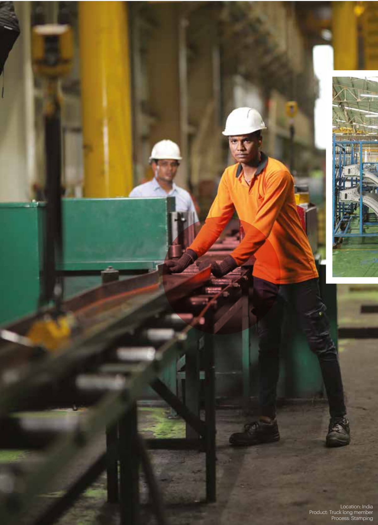
Location: India Product: Truck cabin parts Process: Cabin in white stamping
