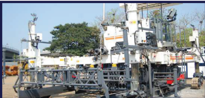
Concret Paver Machine
