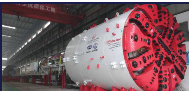
Tunnel Boring Machine (TBM)
