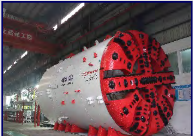
Tunnel Boring Machine (TBM)
