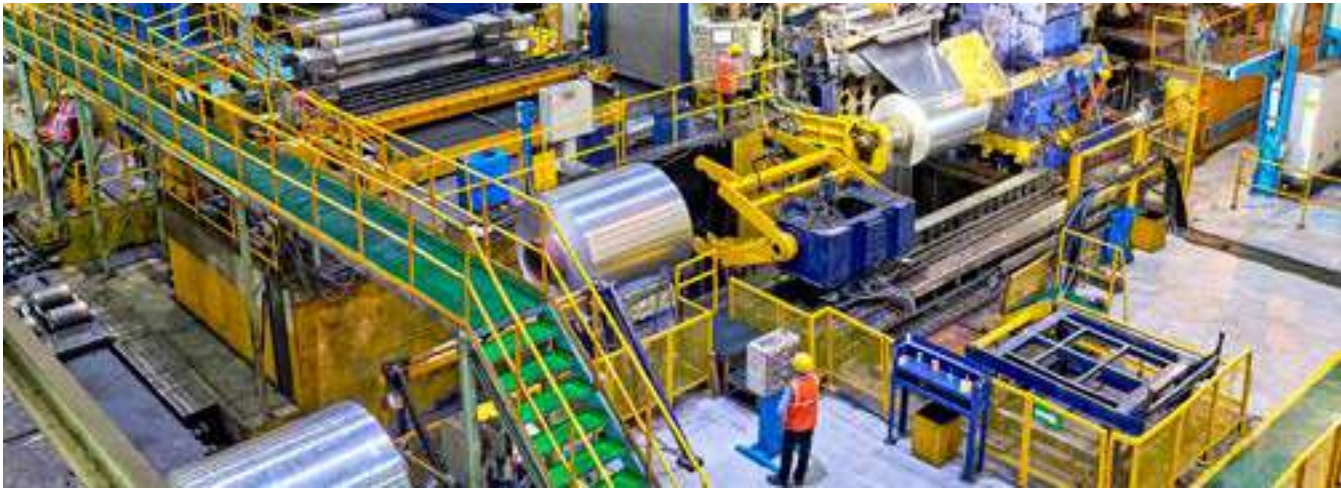
Hirakud FRP- Cold rolling mill operations
