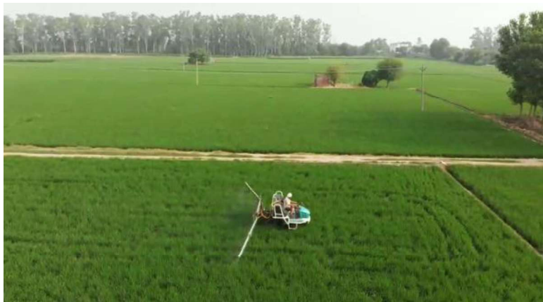
Escorts transplanter-based boom sprayer in action
