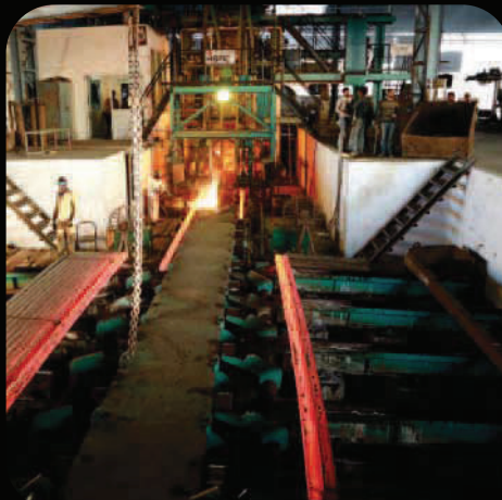
Continuous Casting Machine
