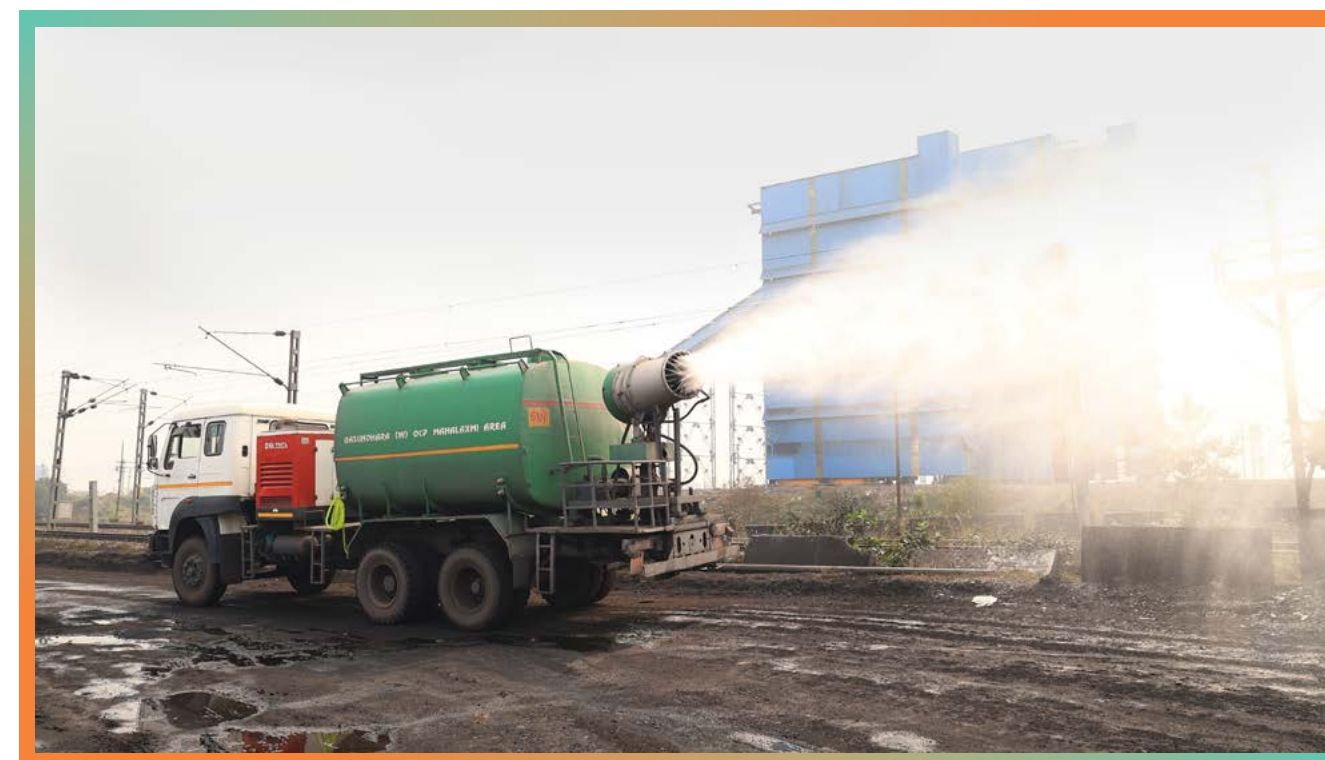
► Fog Cannon for effective dust suppression
