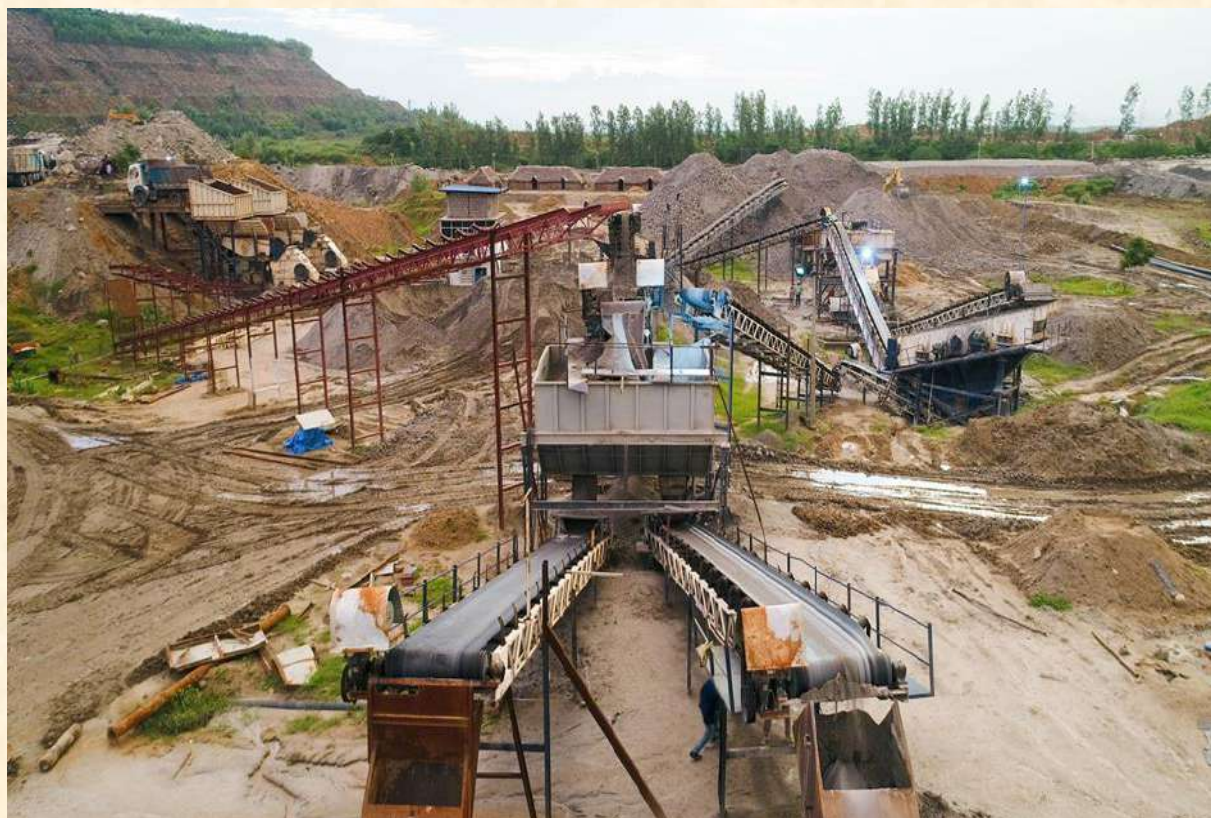
Fig. 50 - OB to sand plant in WCL
