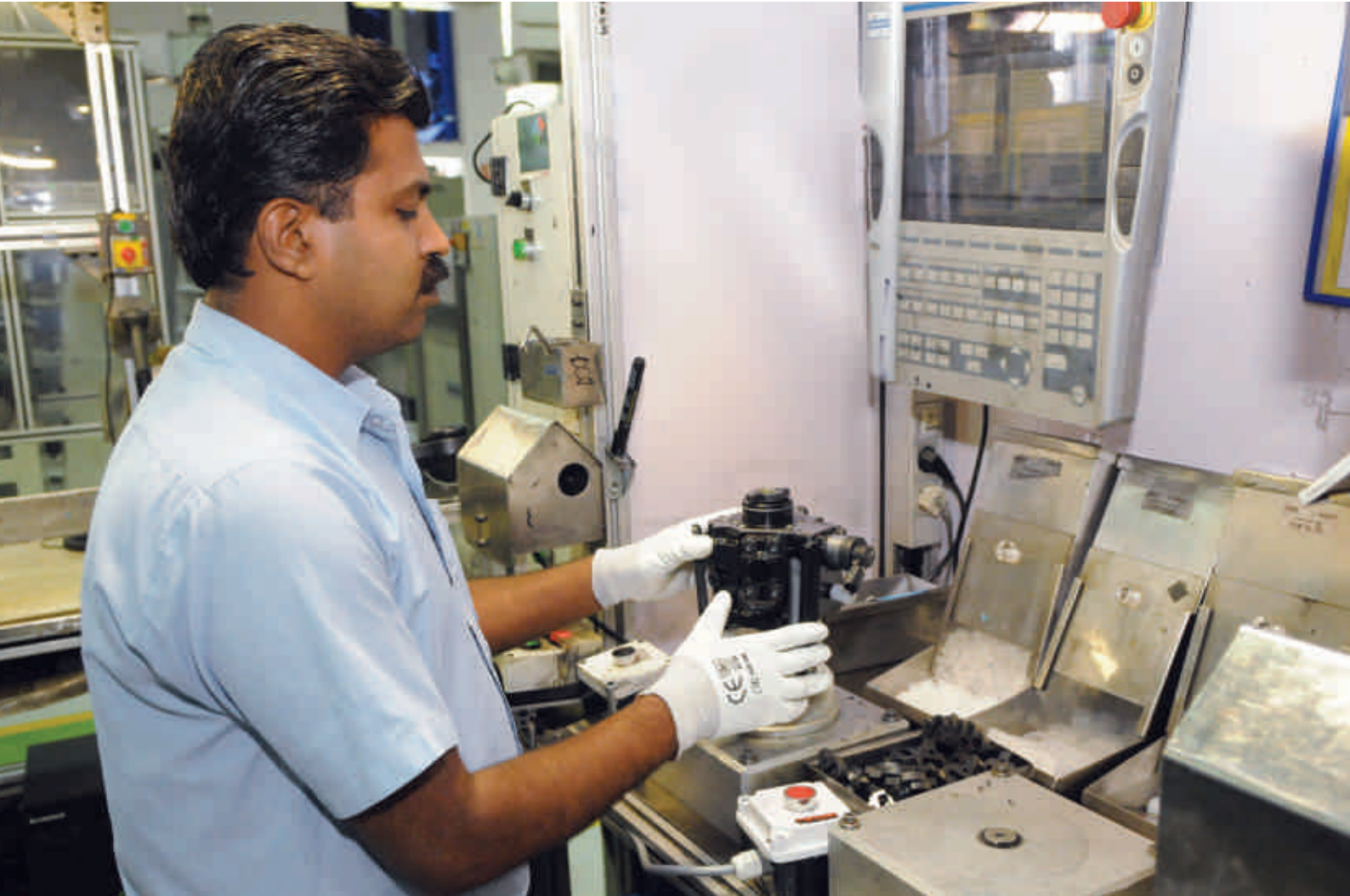
An associate inspecting the Common Rail High Pressure Pump (CP1H).
