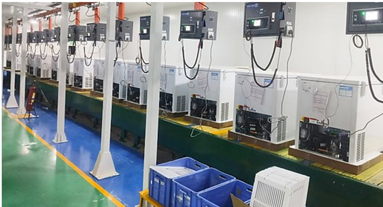
Computerised Performance Testing (CPT) line at Ahmedabad Plant
