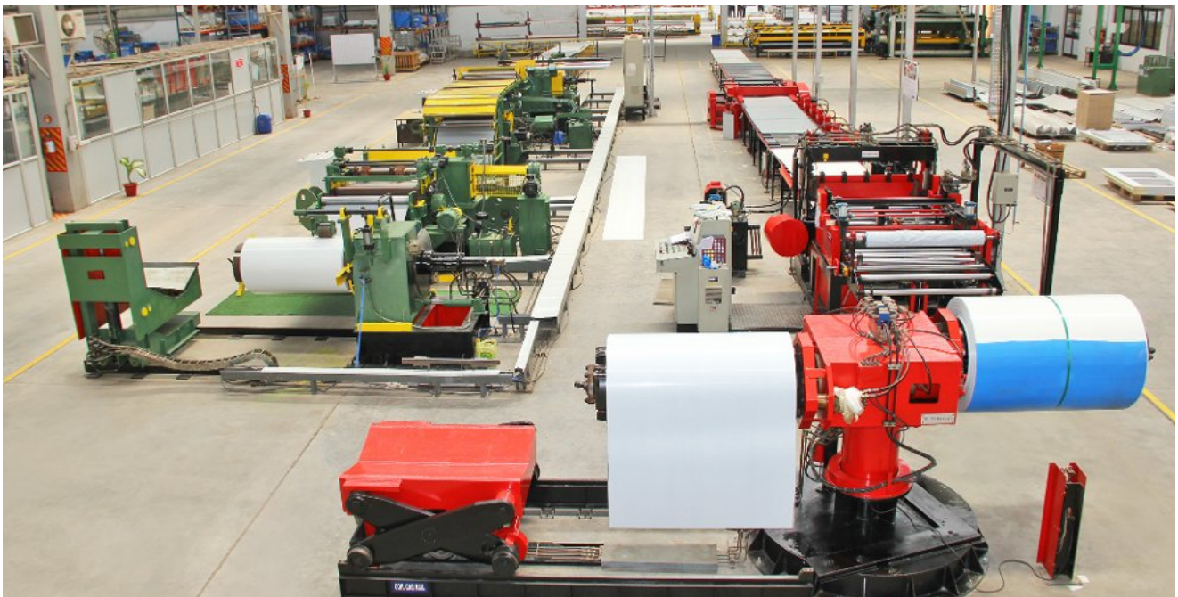
High-capacity insulated panel manufacturing at Wada Plant
