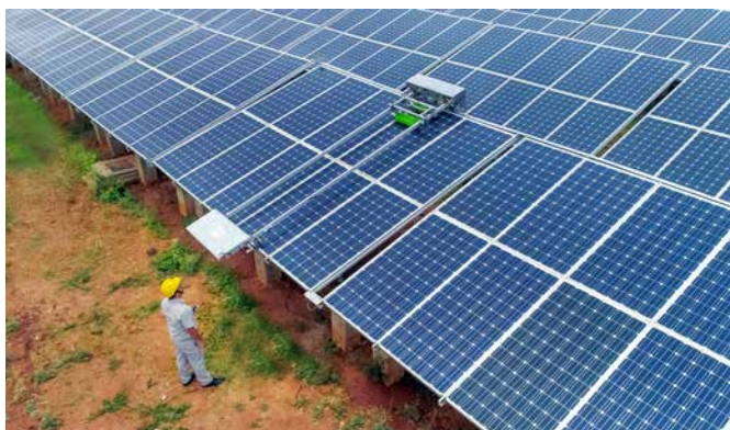
Indigenously developed solar cleaning panel robot under operation at BHEL Corporate R&D, Hyderabad
