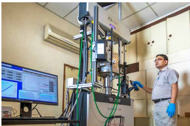
Electromagnetic Resonance Fatigue (ERF) test machine at Corp. R&D, Hyderabad
