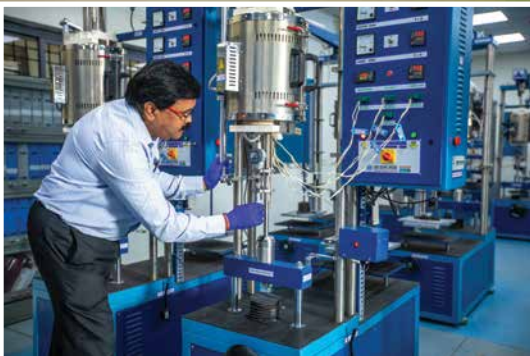
Creep testing of advanced materials for AUSC power plant applications in progress
