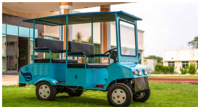
Fuel cell powered 1.25 kW hybrid electric golf cart vehicle developed by BHEL
