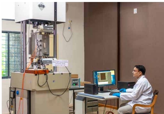
Ambient and high temperature tensile and Low Cycle Fatigue (LCF) test facility for metallic materials at Corp. R&amp;D, BHEL Hyderabad
