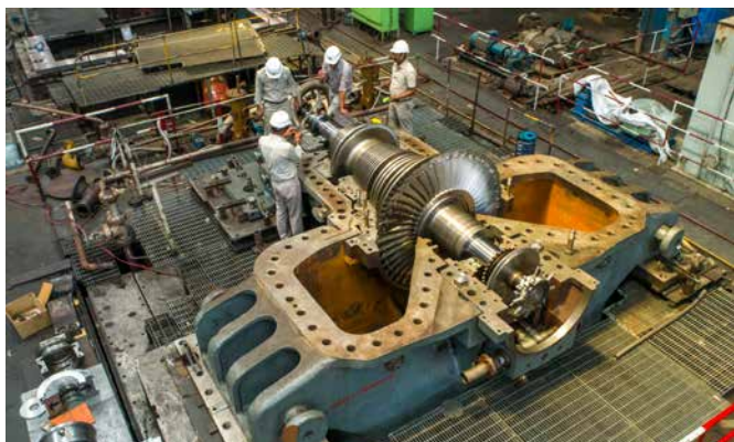
150 MW steam turbine for captive power plant at BHEL works at Hyderabad
