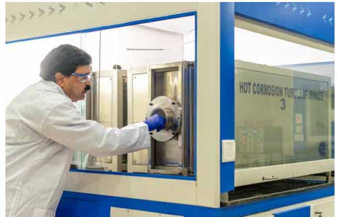
Furnaces for testing fire side corrosion of alloys and welds at Corp. R&D, Hyderabad
