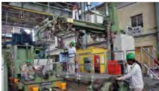
Welding overlay machine at BHEL, Haridwar
