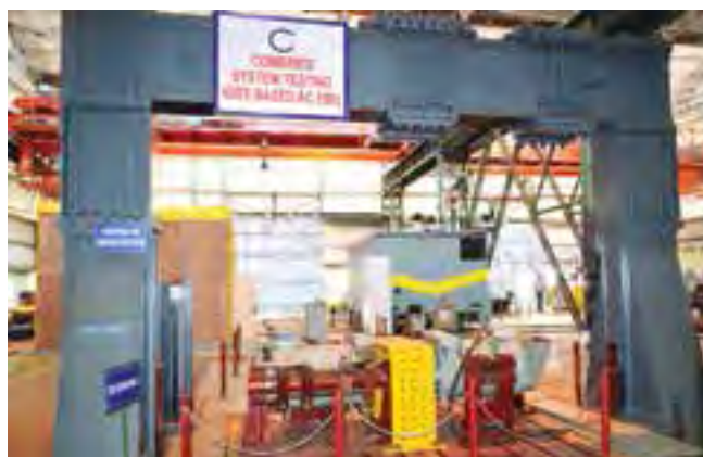
Combined System Testing for IGBT-based AC EMUs at Centre for Electric Transportation at BHEL, Bhopal
