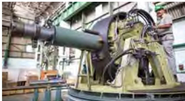
Super Rapid Gun Mount (SRGM) for Indian Naval Ships under assembly at BHEL, Haridwar
