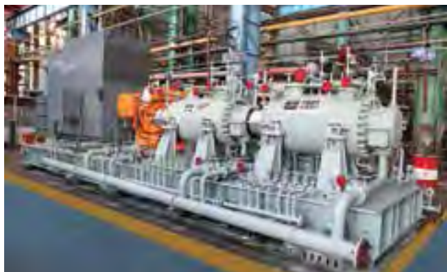
Centrifugal compressor under assembly at BHEL works in Hyderabad
