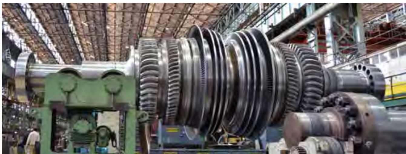
800 MW LP rotor under assembly at BHEL, Haridwar
