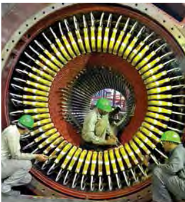
Stator manufacturing under progress at BHEL, Haridwar
