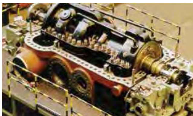
New back-pressure HP module for two-cylinder reheat steam turbine, under assembly at BHEL works, Hyderabad
