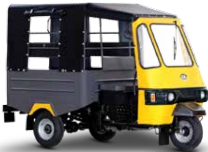
FRONT ENGINE | PASSENGER 6+1 500 KG PAYLOAD CAPACITY
